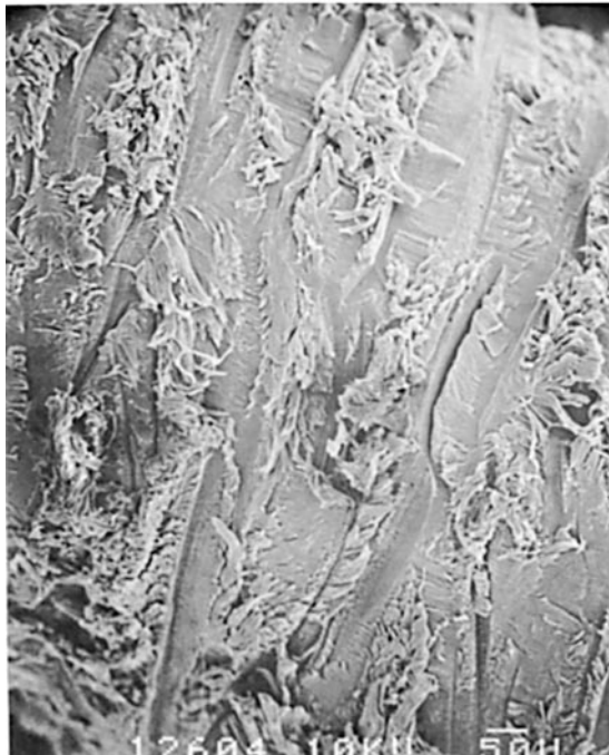
Figure 2 SEM micrographs of the POM fiber surfaces treated with HFP: (a) the fiber surface after the immersion of the intact fiber in HFP for 7 days at room temperature, (b) the surface of the fiber that was immersed in HFP for 3 min after sandpapering using 40 mesh, and (c) higher magnification of (b).
